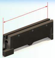
Face Width:- This is the width of the sealed area on the package.
